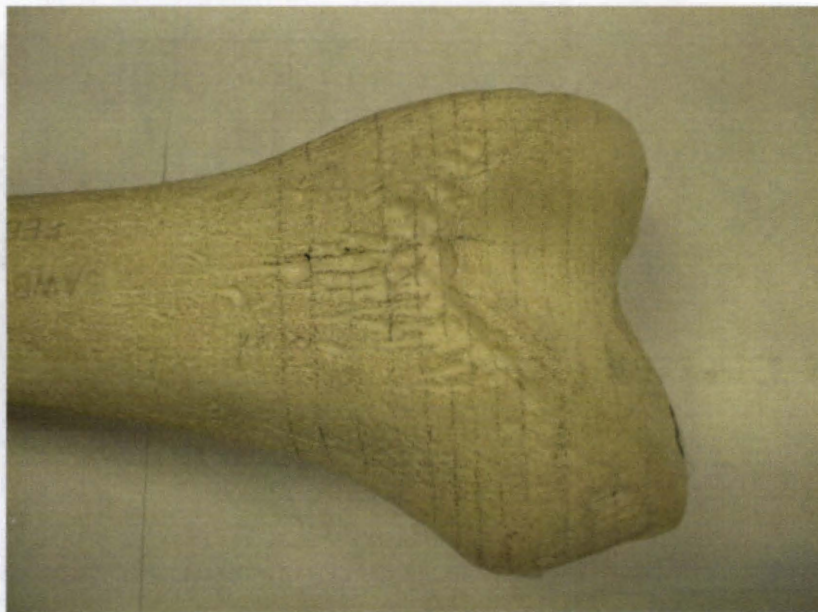
Figure A6: Section Markings on Sawbones
