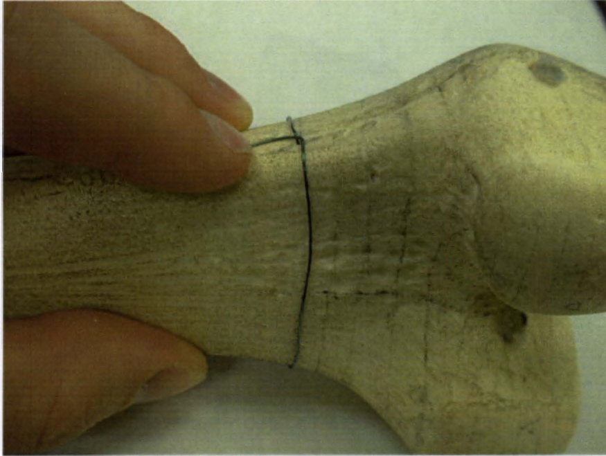
Figure A7: Applying Magnet Wire to Sawbones
